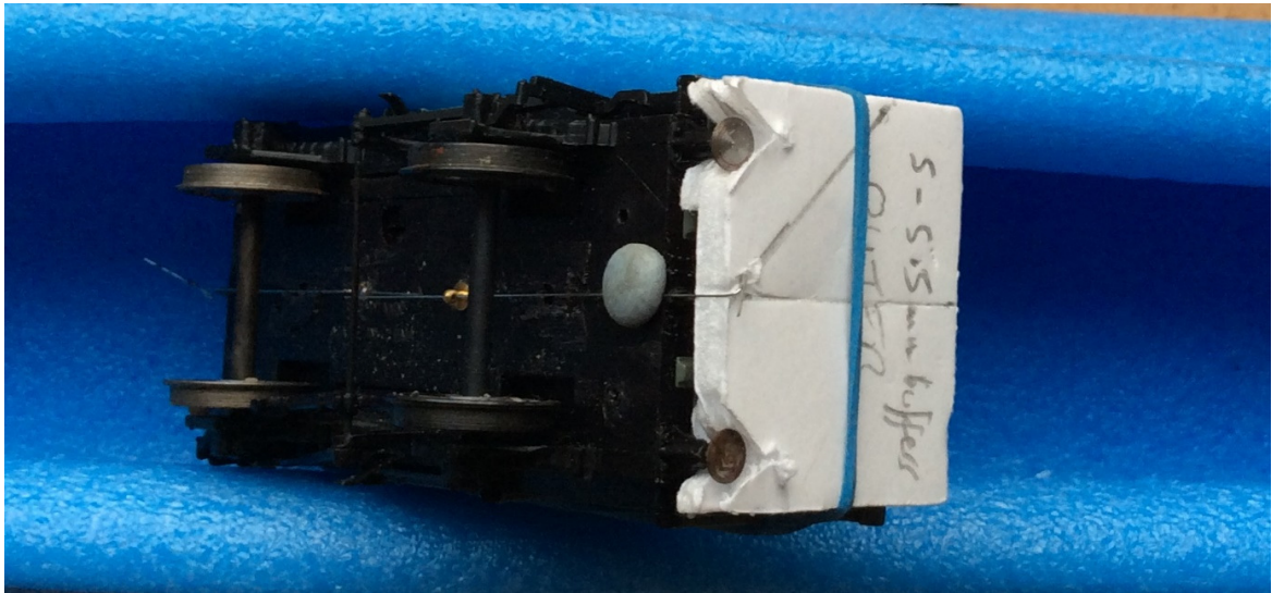
Jig held in place by rubber band and buffers. Coupling held in place by jig, by Blutak on buffer beam and handrail knob. Hook and nose are aligned with the 45° line on the jig.
