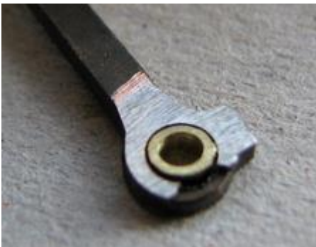
Photo 63 - Connecting rod bushes in place - as a running fit!
