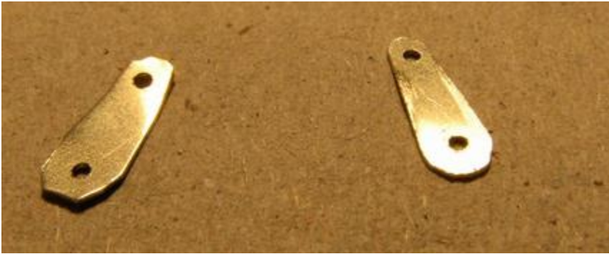
Photo 52 - shows one crank cut out by tin snips and the second has been filed up neatly and straightened out with pliers.
