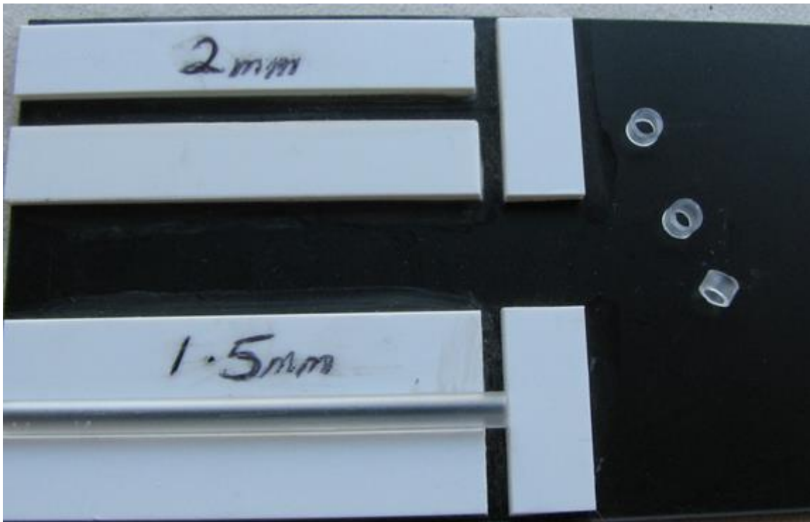
Photo 30 - These are cut from the empty inner ink holding tube of a biro. Slice off spacers, 1.5mm approx in width, and we need 4 for the bogie, 2 per axle.
