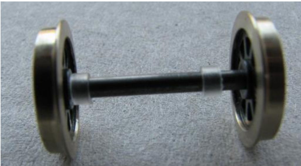
Photo 31 - One assembled EM bogie wheel set, incorporating two of our biro spacers.
