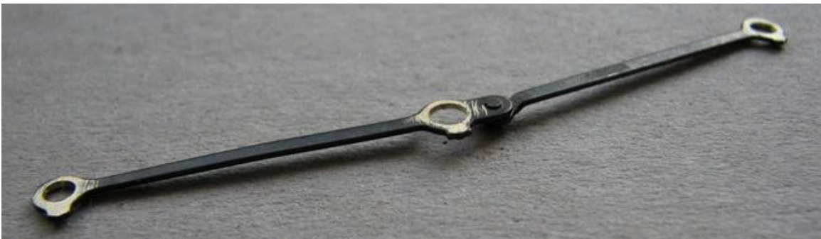
Photo 56 - original coupling rods - un-bushed - holes too big.
