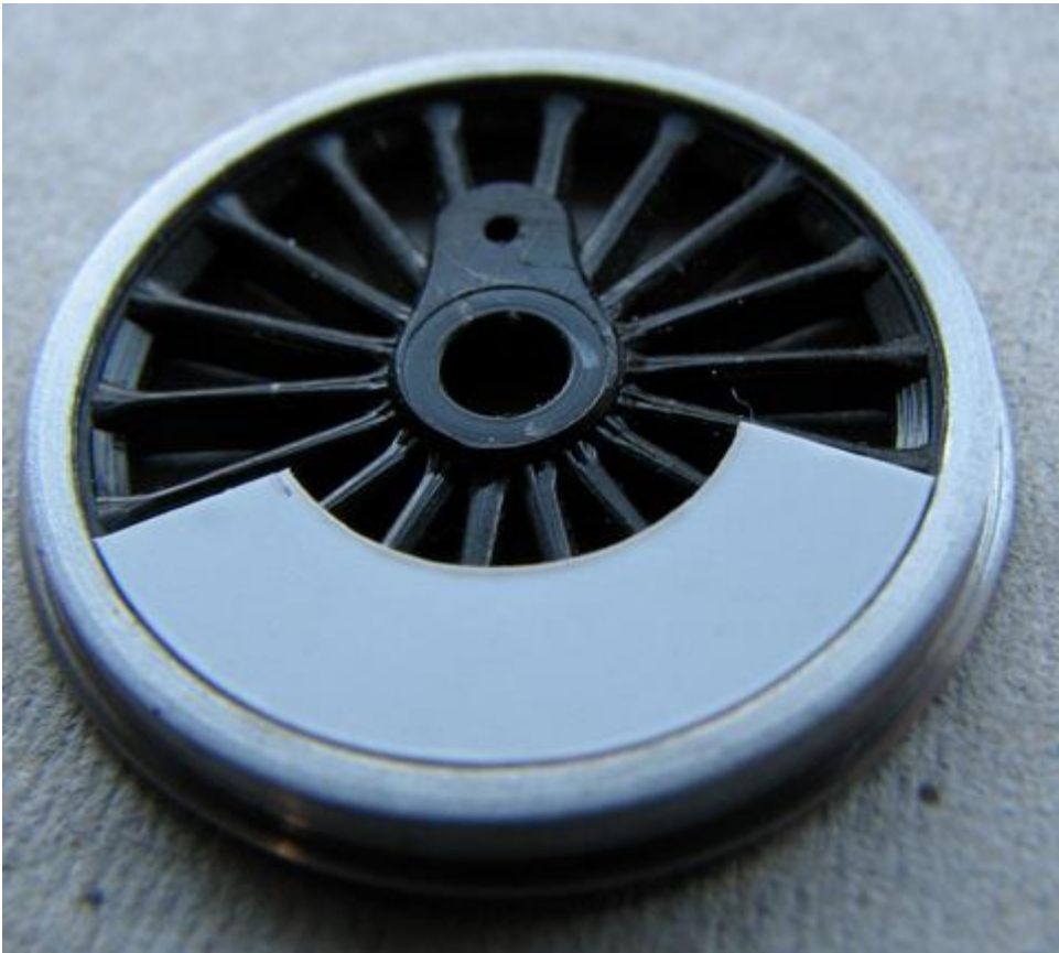
Photo 38 - shows close up of centre axle wheel balance weight
