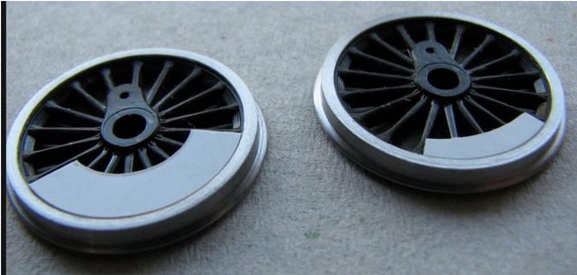
Photo 36 - shows the fitted balance weights
