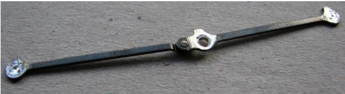
Photo 59 - Coupling rods with bushes soldered in place. You will fill in the holes more likely than not,
