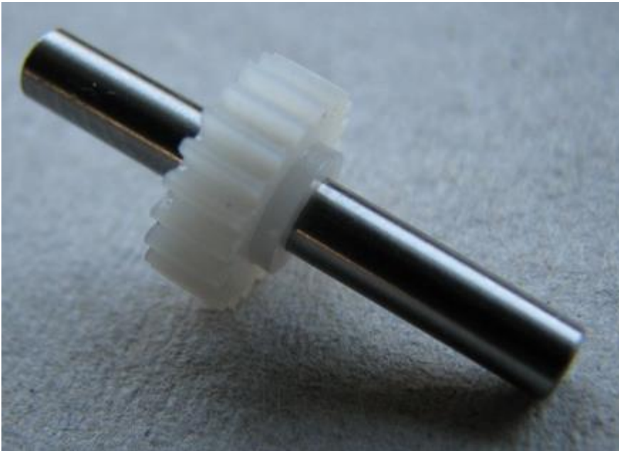
Photo 39 - The gear wheel is fitted to one axle, using Loctite 601 to ensure it remains in position. The gear needs to be 10mm from the face of the gear boss to the axle end. Leave to cure, and make sure any excess Loctite is removed!
