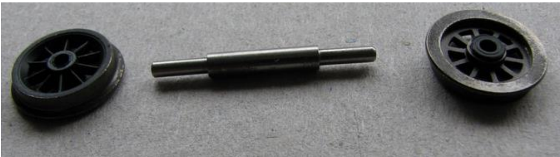
Photo 8 - Bachmann axle showing the 2mm shoulders, with the Bachmann wheels removed - simply twist them off whilst holding the axle firmly with pliers, or tap the axle through whilst supporting the back of the wheel over the slightly open jaws of a vice.
