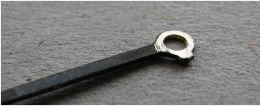
Photo 57 - Simply file the rod rear face until the plating is removed to expose clean metal.
