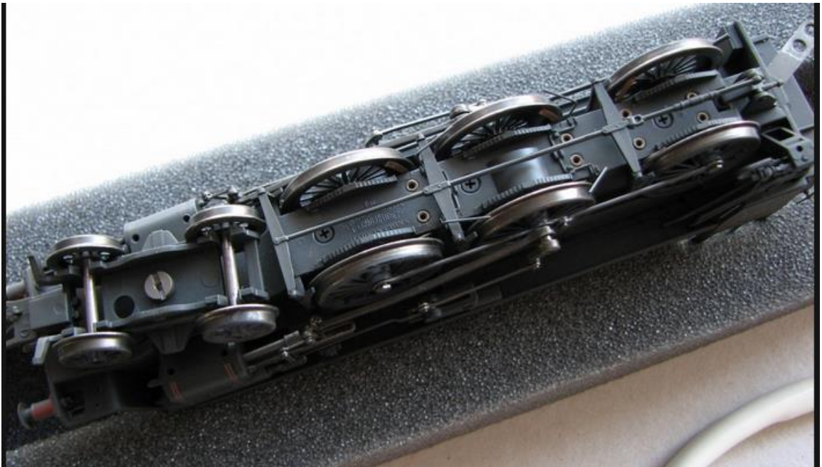
Photo 14 - the underside view of the loco, showing the brake gear which needs removing. Incidentally, the cradle the loco is sitting in is the Peco Loco Servicing cradle. I am always being asked that!
