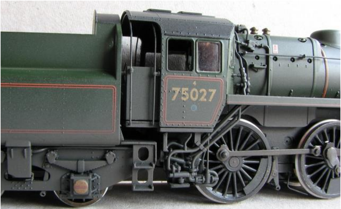
Photo 75 - A much closer engine / tender coupling. It will negotiate pretty tight curves at this spacing!
