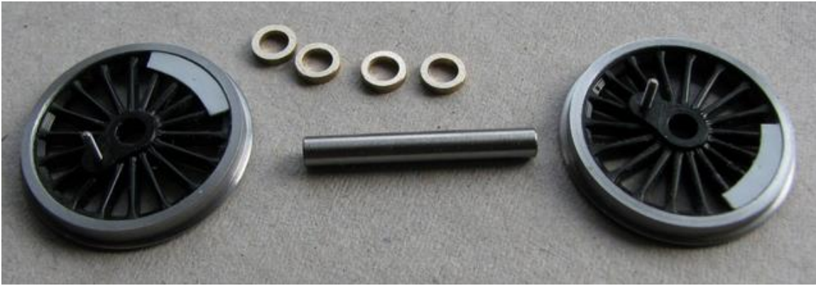
Photo 40 - Wheel set assembly. This picture shows the spacers needed on axles to limit side play.
