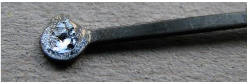
Photo 60 - but notice that the solder forms a neat depression in the centre of what was the hole. This is used as a centre punch mark to drill out the hole. Using a
