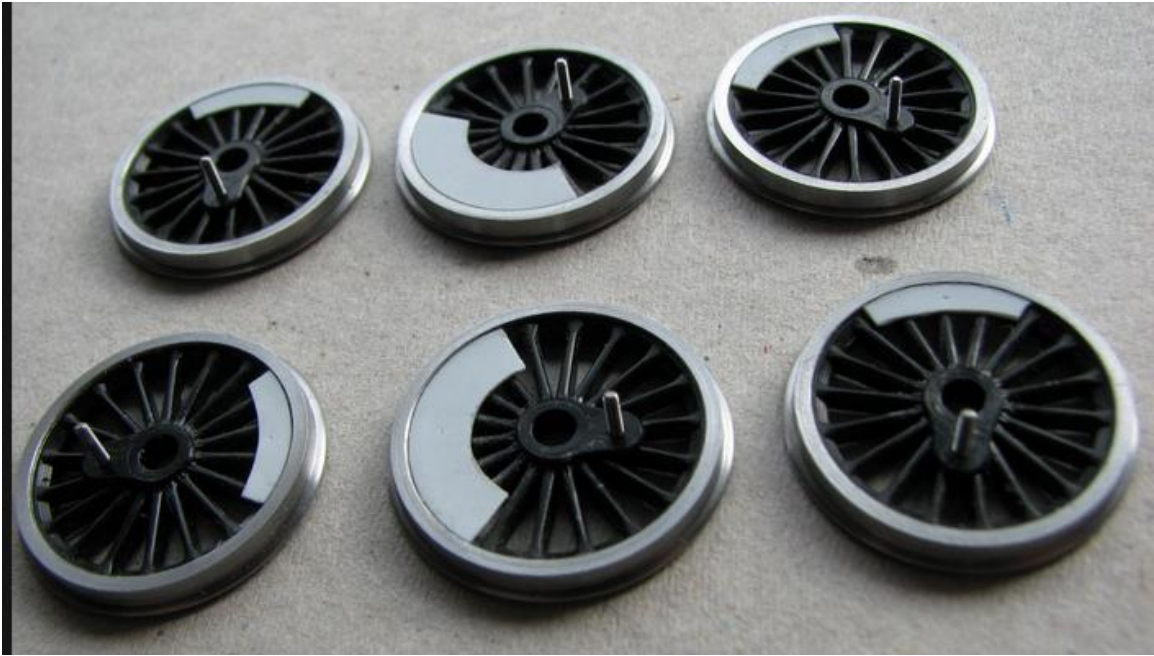
Photo 37 - the complete set with the crankpins fitted to the 6 driving wheels. Follow the Alan Gibson instructions supplied with their crankpins for this step.
