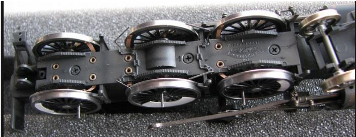
Photo 45 - Replace keeper plate ensuring it is aligned the correct way round and that the pickups align with the rear of the steel wheel-treads.
