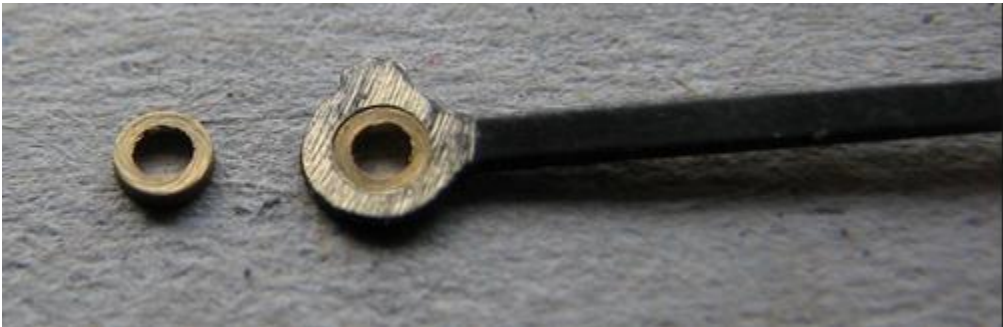
Photo 58 - Also, twist a round needle file anti clockwise in each hole just sufficient so that the Gibson bushes, or 14BA washers can be pushed in and so that the inside of the hole is clean metal for soldering the bush in place. Solder the bushes/washers into the rods as per Photo 59 below.
